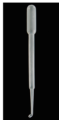
图1 用于平铺密度梯度分离体系的弯头塑料滴管 Fig.1 Curving plastic dropper used to build density gradient separation system
